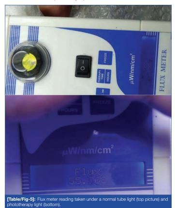
A five point measurement of flux was taken from all four corners and the centre of the phototherapy unit bed (where the baby was positioned for phototherapy) and the average of these five readings was taken for calculating flux. In accordance with the AAP chart, the decision to stop phototherapy was based on a reduction in serum bilirubin to below the phototherapy range [4].
